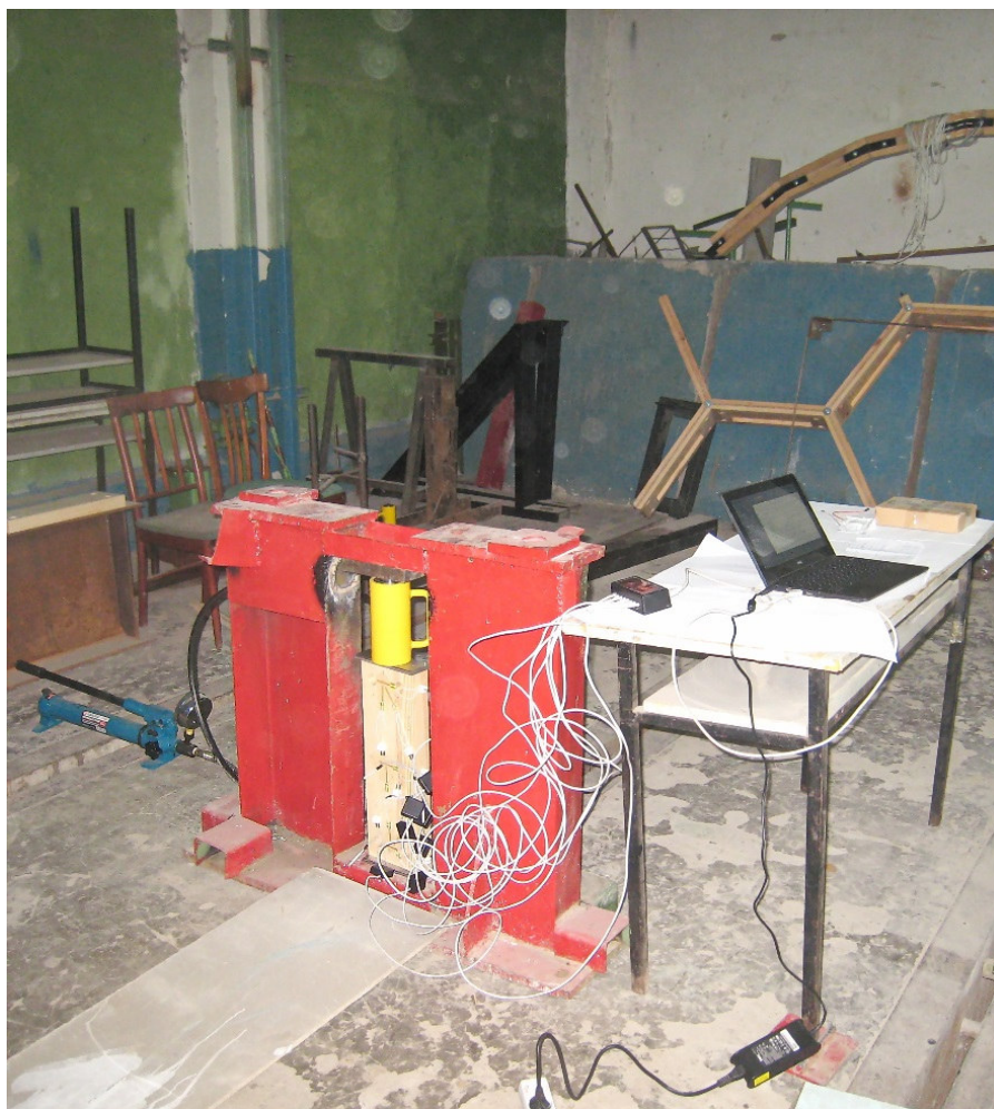
Fig. 1. Test bench for compression testing of glued wood samples
